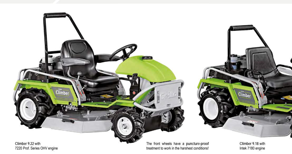
The Climber model 9.22 is fitted with an Intek 7220 Prof. Series 18 HP (22 HP Gross Power) engine, has a comfort seat with armrests, tall roll bar. The 9.18 model is fitted with an Intek 7180 15.2 HP (18 HP Gross Power) engine, damped seat, low roll bar.
