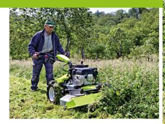
The CL 75 is fitted with a GXV 390 petrol engine. The single-cylinder engine has a displacement of 389 cc and features state-of-the-art technology to ensure reliability such as overhead valves, low emissions, low fuel consumption, high performance and minimal vibration.
