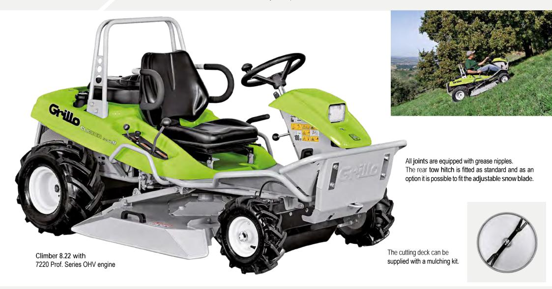
The Climber 8.22 is fitted with a 7220 Professional Series, 18 HP (22 HP Gross Power) petrol engine with 7 L tank and level indicator on the cap. The two-cylinder engine with overhead valves and cast iron cylinders has a displacement of 656 cc and features state-of-the-art solutions that ensure reliability, low emissions, low fuel consumption, high performance and minimal vibrations.
