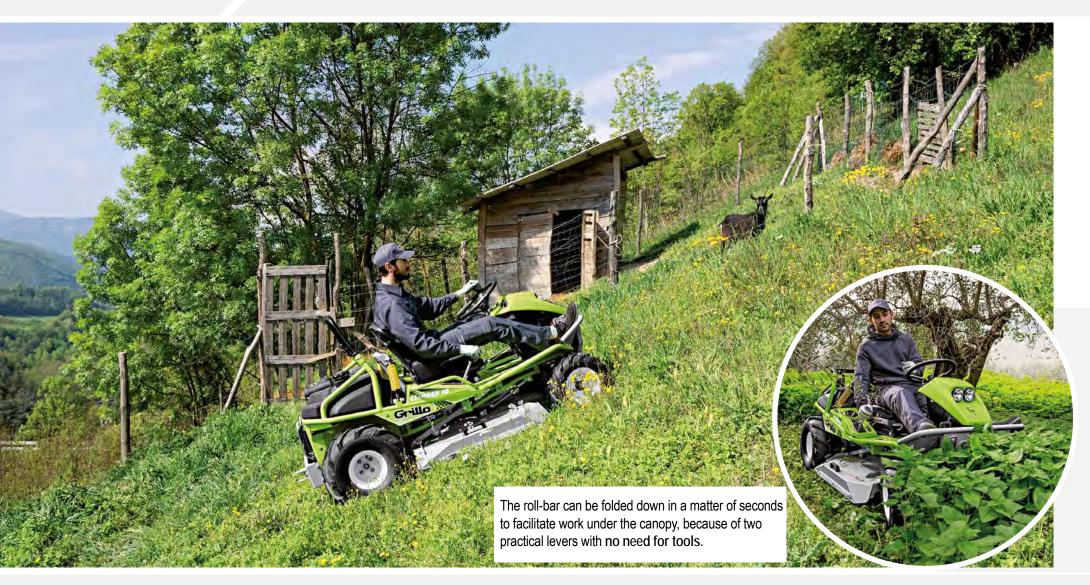
Fast transfers with a maximum speed of 9 km/h. In case of very uneven terrain it is possible to raise the cutting deck up to 13.5 cm from the ground.
