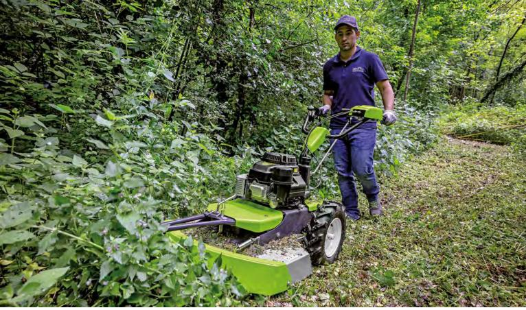
The CL 62M is fitted with a OHV single cylinder petrol engine, 179 cc, 4.5 HP with a 1.6 L fuel tank and forced lubrication system, allowing the machine to work on slopes up to 30°.
