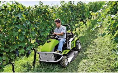
The extremely small turning radius of only 38 cm allows to move in tight areas.
