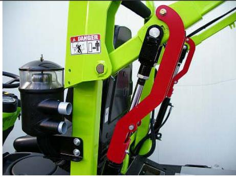
**CAUTION!** When making the engine maintenance and keeping the grass catcher up, engage the two red safety lockings on the hydraulic cylinders. Do not work on the engine without having engaged the lockings. Do not keep the machine stopped with the grass catcher up without having engaged the two red safety lockings.
