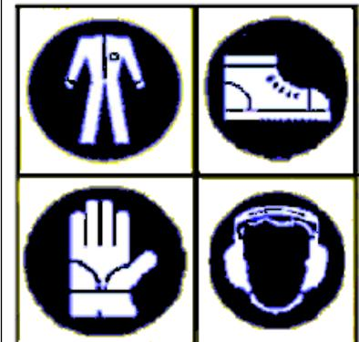
Before using the machine, it is mandatory to put on the appropriate individual safety devices: body protection, protection gloves, security shoes, ear protection.
