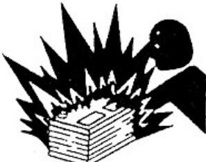
*Prevent battery explosions: keep sparks, lighted matches, and open flame away from the top of battery. Battery gas can explode.*
