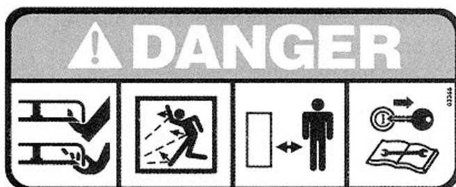
**WARNING!** SHARP PARTS. Keep hands and feet away. Do not operate the mower over gravel or foreign bodies which may be sucked up and ejected by the blades, generating a danger. Keep people away. remove the key and read the instruction manual before attempting to carry out any maintenance or repairs to the machine.
