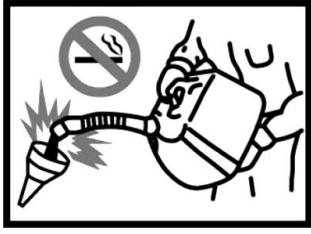
Handle fuel with care, it is highly flammable: Do not refuel machine while smoking, when machine is near an open flame or sparks, or when the engine is running. Stop the engine.
