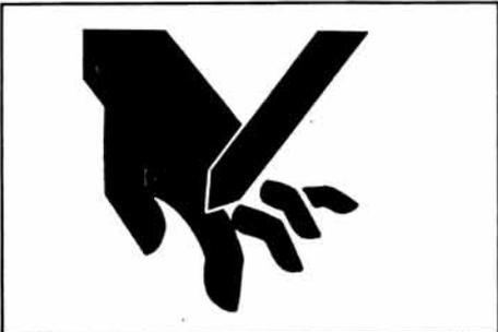
*Sharp component. Keep hands and feet away do not clean the attachment when the engine is turning.*
