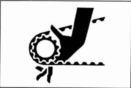
*Caution! Never touch moving pulleys or belts. They can be very dangerous. Never carry out maintenance with engine running.*
