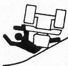
*Avoid Tipping. Do not drive where machine could slip or tip. Stay alert for holes and other hidden.*
