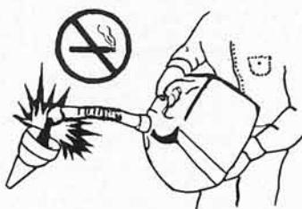
*Handle fuel with care, it is highly flammable: Do not refuel machine while smoking, when machine is near an open flame or sparks, or when engine is running. Stop engine.*
